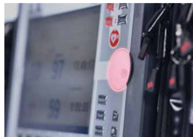
▲ Alarm visualization via glowing JogDial as well as warning tones.
